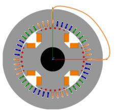
Figure 2: Full pitch winding
