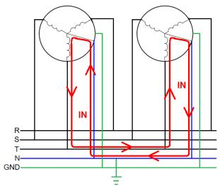
Figure 7: Circulating neutral current
