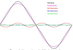
Figure 6: Harmonics with 5/6 pitch winding
