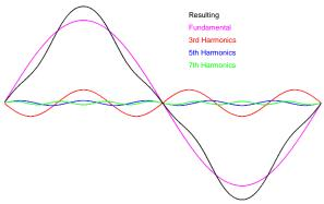
Figure 1: Relation between waveform and harmonics
