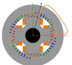
Figure 3: Fractional pitch winding (5/6)
