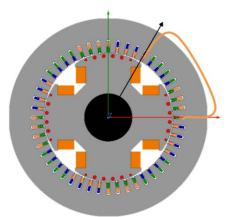
Figure 4: Fractional pitch winding (2/3)
