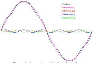
Figure 5: Harmonics with 2/3 pitch winding
