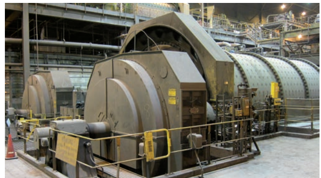
United Taconite LLC - Minnesota USA Dual Pinion SAG Mill - 2x LSS Motor + Airclutch Load Sharing System
